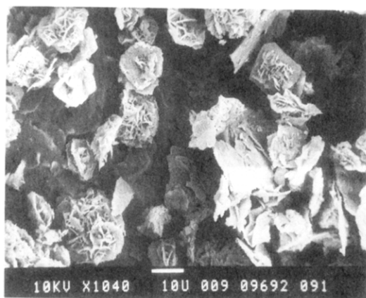
Figure 6. SEM micrograph of poly(ester-imide) 6a prepared from monomer 4b (silyl method) at 400 °C/4 h.
